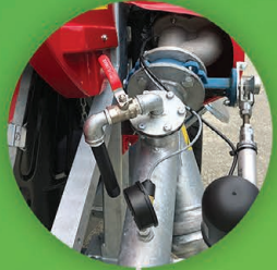
Water Inlet Drain Valve
